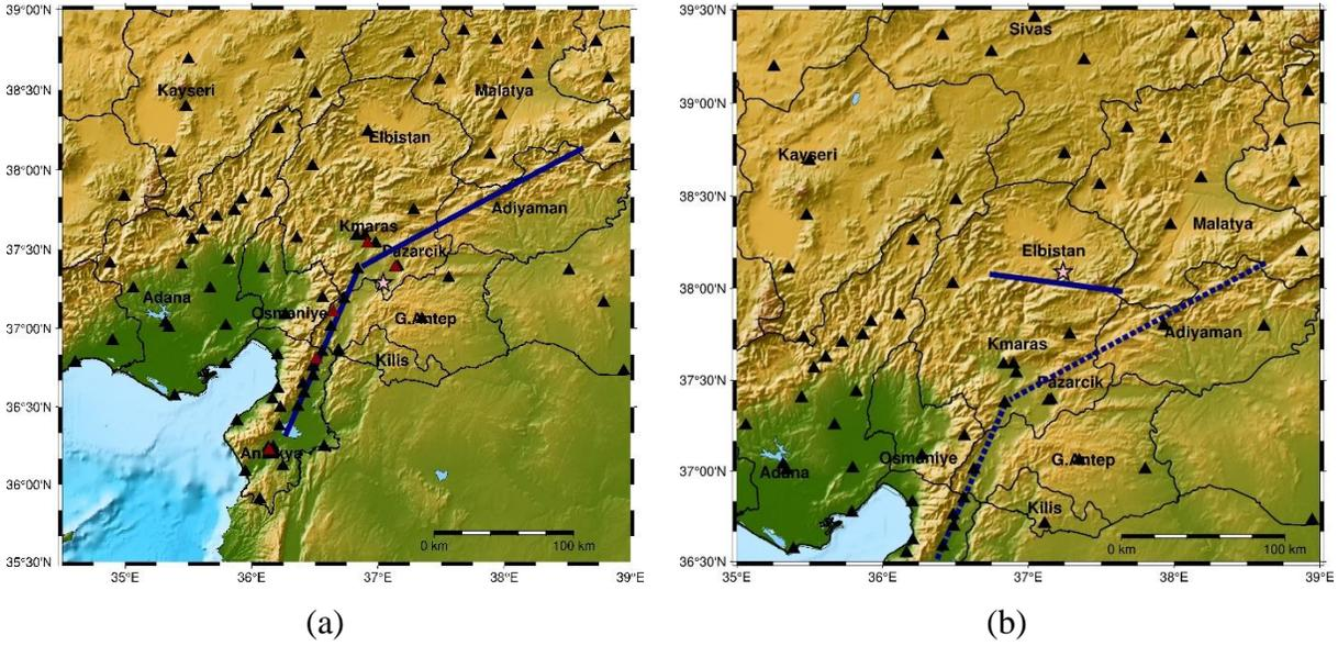
**Figure 4.5.** Distribution of the strong motion stations that are located within 200km of the rupture plane for (a)  $M_w=7.7$  Kahramanmaraş-Pazarcik and (b)  $M_w=7.5$  Elbistan earthquakes.
