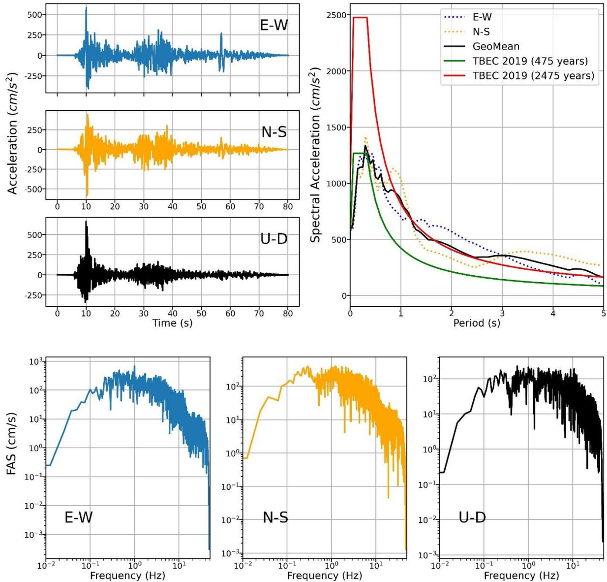
**Figure 4.11.** Recorded three-component ground accelerations, corresponding Fourier amplitude spectra (FAS) and response spectra (with 5% damping) in comparison with the most recent building code (TBEC, 2019) at selected station 4615 due to Pazarcik ( $M_w=7.7$ ) event
