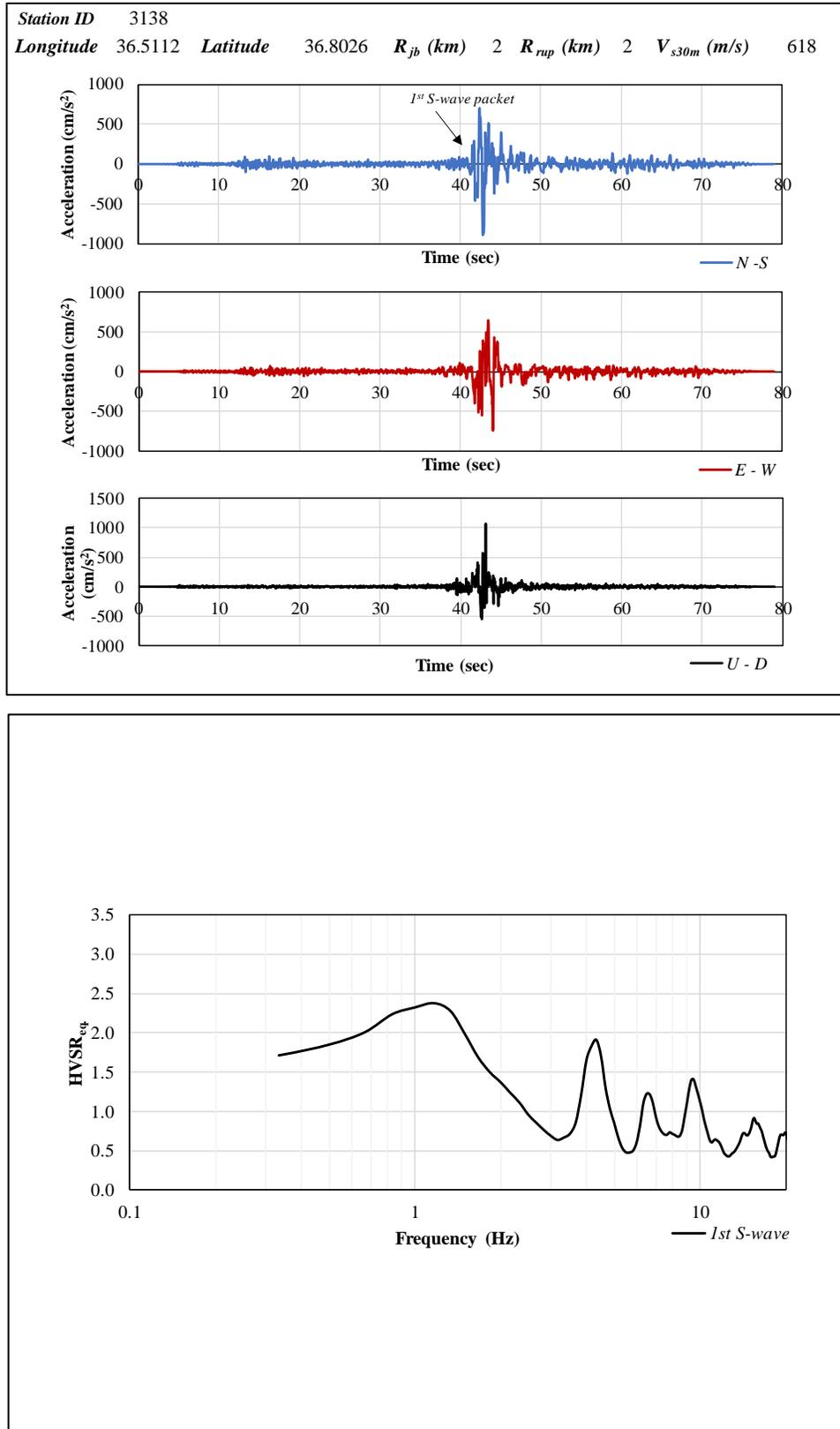
Figure 4.29. Resulting HVSR curve for station 3138
