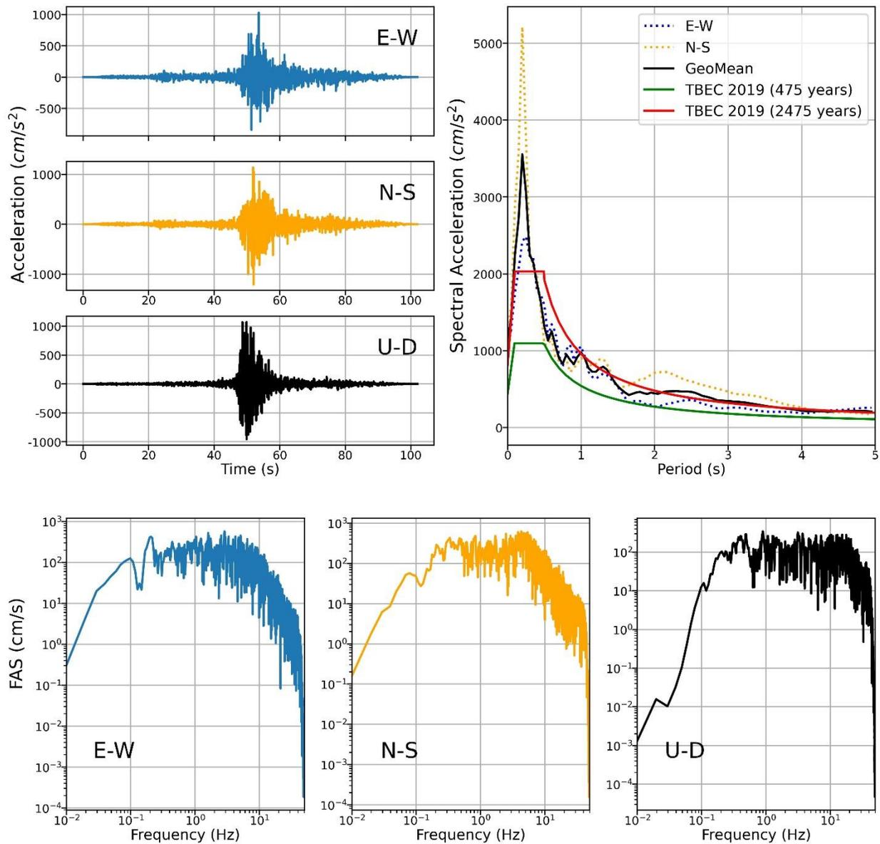
**Figure 4.9.** Recorded three-component ground accelerations, corresponding Fourier amplitude spectra (FAS) and response spectra (with 5% damping) in comparison with the most recent building code (TBEC, 2019) at selected station 3126 due to Pazarcik ( $M_w=7.7$ ) event
