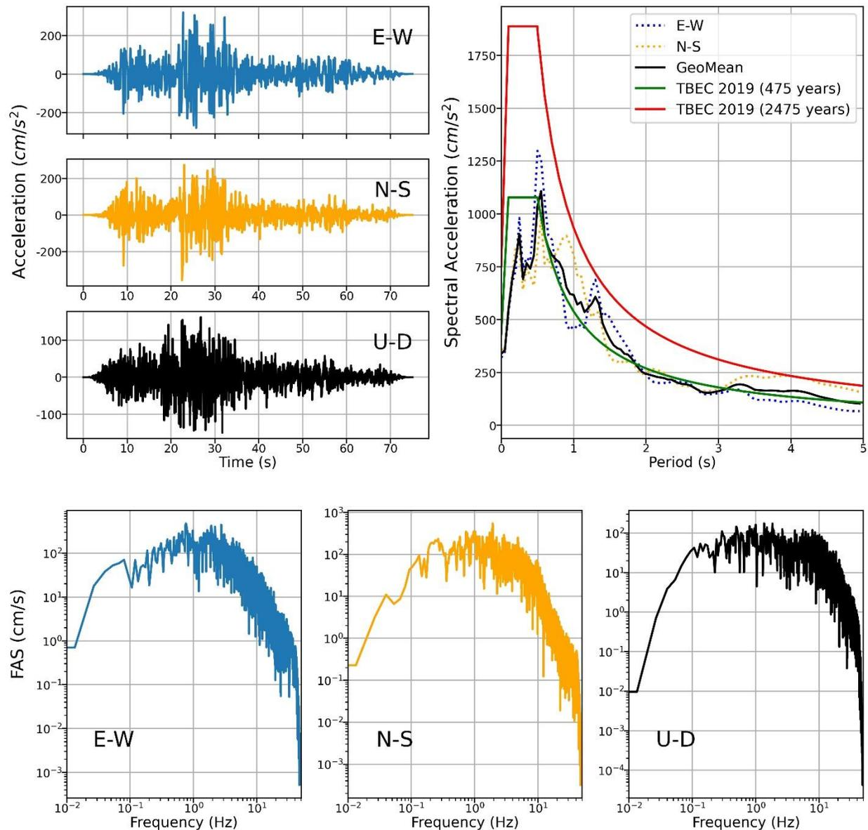
**Figure 4.12.** Recorded three-component ground accelerations, corresponding Fourier amplitude spectra (FAS) and response spectra (with 5% damping) in comparison with the most recent building code (TBEC, 2019) at selected station 4624 due to Pazarcik ( $M_w=7.7$ ) event
