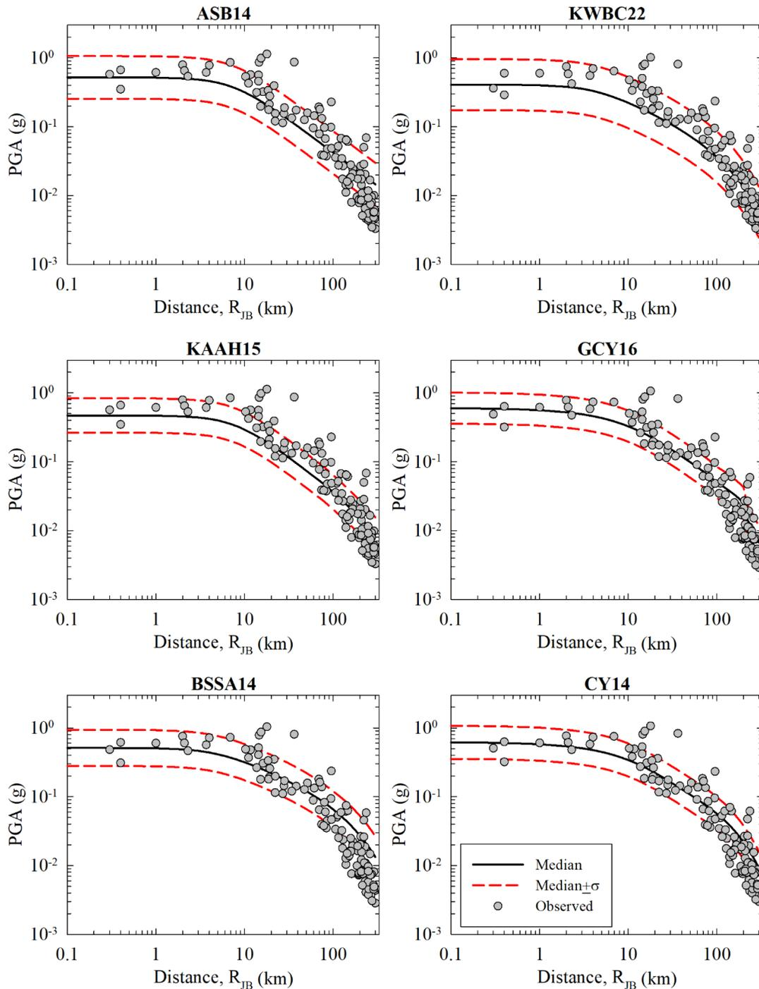
**Figure 4.17.** Comparison of the distance attenuation of ASB14, KWBC22, KAAH15, GCY16, BSSA14, and CY14 models with recorded strong motion data for PGA. Median and median  $\pm 1\sigma$  curves are given with black solid and red dashed lines, respectively. Gray points represent the  $V_{S30}$  normalized recorded strong motion data for Pazarcik Earthquake.
