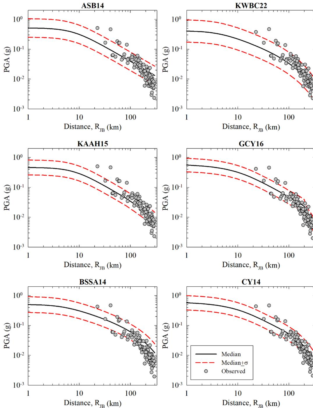
**Figure 4.22.** Comparison of the distance attenuation of ASB14, KWBC22, KAAH15, GCY16, BSSA14 and CY14 models with recorded strong motion data for PGA. Median and median  $\pm 1\sigma$  curves are given with black solid and red dashed lines, respectively. Gray points represent the  $V_{S30}$  normalized recorded strong motion data for Elbistan Earthquake.
