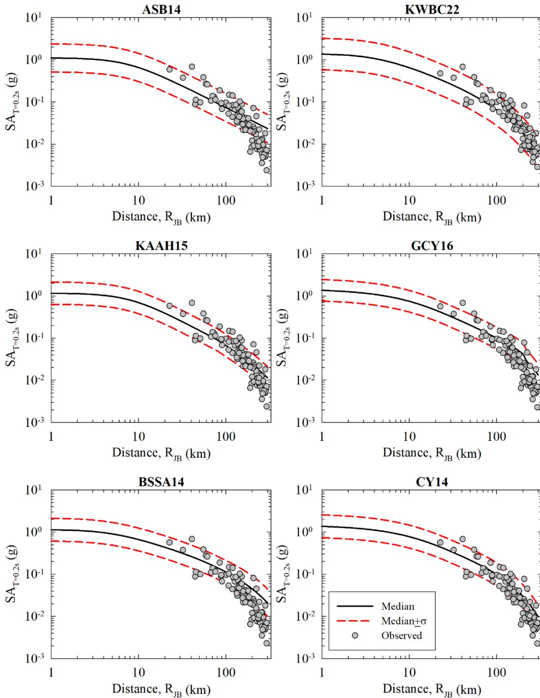
**Figure 4.24.** Comparison of the distance attenuation of ASB14, KWBC22, KAAH15, GCY16, BSSA14 and CY14 models with recorded strong motion data for  $T=0.2s$  PSA. Median and median  $\pm 1\sigma$  curves are given with black solid and red dashed lines, respectively. Gray points represent the  $V_{S30}$  normalized recorded strong motion data for Elbistan Earthquake.
