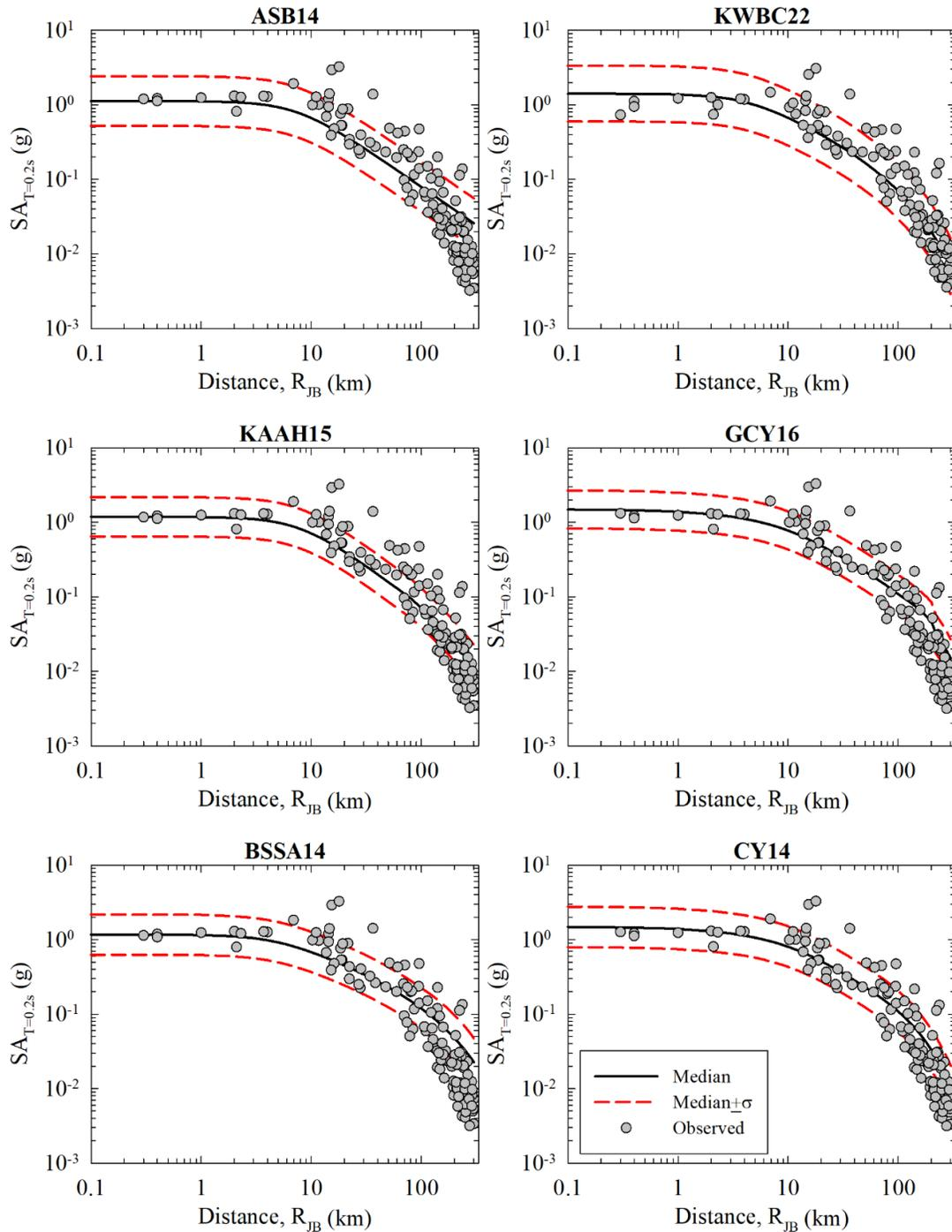
**Figure 4.19.** Comparison of the distance attenuation of ASB14, KWBC22, KAAH15, GCY16, BSSA14, and CY14 models with recorded strong motion data for  $T=0.2s$  PSA. Median and median  $\pm 1\sigma$  curves are given with black solid and red dashed lines, respectively. Gray points represent the  $V_{S30}$  normalized recorded strong motion data for Pazarcik Earthquake.
