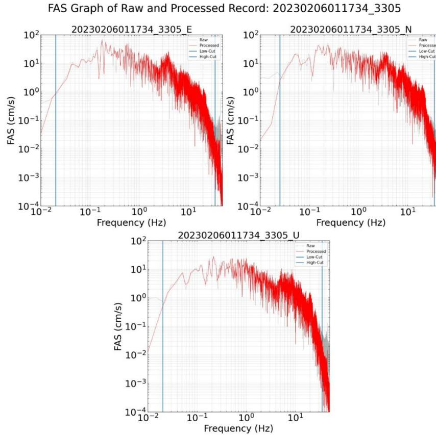
**Figure 4.4.** FAS of the raw and processed waveforms. The blue solid lines show the low- and high-cut filter frequencies.
