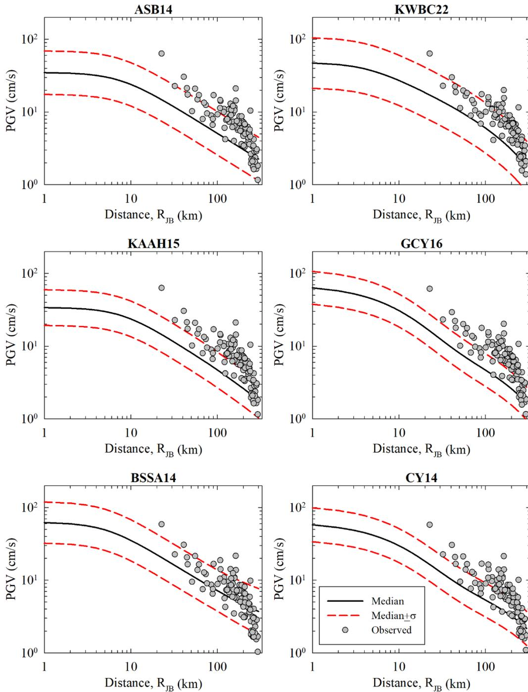
**Figure 4.23.** Comparison of the distance attenuation of ASB14, KWBC22, KAAH15, GCY16, BSSA14 and CY14 models with recorded strong motion data for PGV. Median and median  $\pm 1\sigma$  curves are given with black solid and red dashed lines, respectively. Gray points represent the  $V_{S30}$  normalized recorded strong motion data for Elbistan Earthquake.
