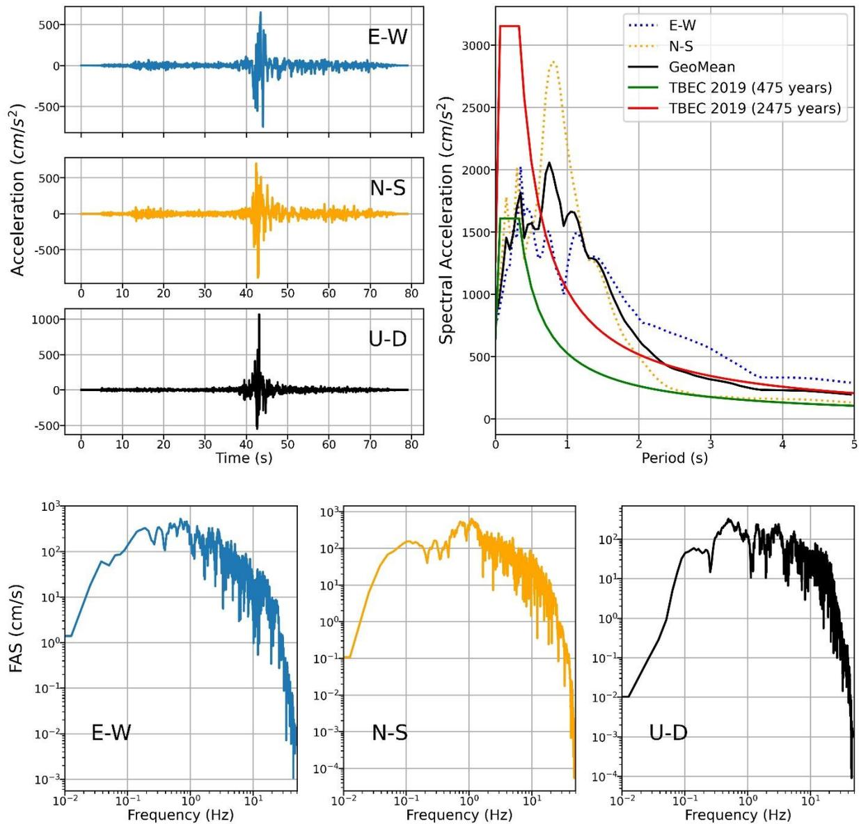
**Figure 4.10.** Recorded three-component ground accelerations, corresponding Fourier amplitude spectra (FAS) and response spectra (with 5% damping) in comparison with the most recent building code (TBEC, 2019) at selected station 3138 due to Pazarcik ( $M_w=7.7$ ) event
