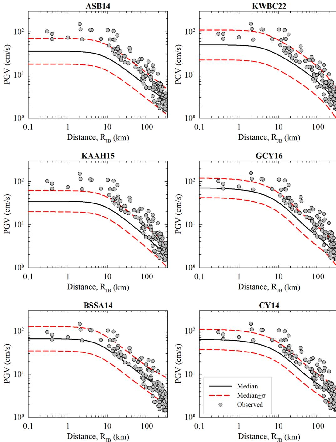
**Figure 4.18.** Comparison of the distance attenuation of ASB14, KWBC22, KAAH15, GCY16, BSSA14, and CY14 models with recorded strong motion data for PGV. Median and median  $\pm 1\sigma$  curves are given with black solid and red dashed lines, respectively. Gray points represent the  $V_{S30}$  normalized recorded strong motion data for Pazarcik Earthquake.
