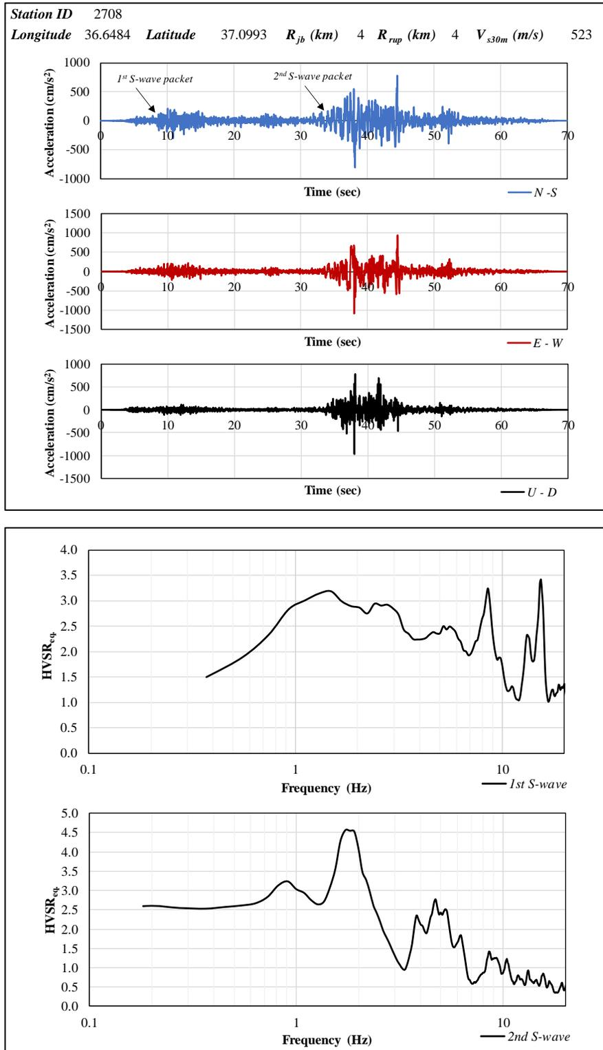
**Figure 4.27.** Resulting HVSR curve for station 2708
