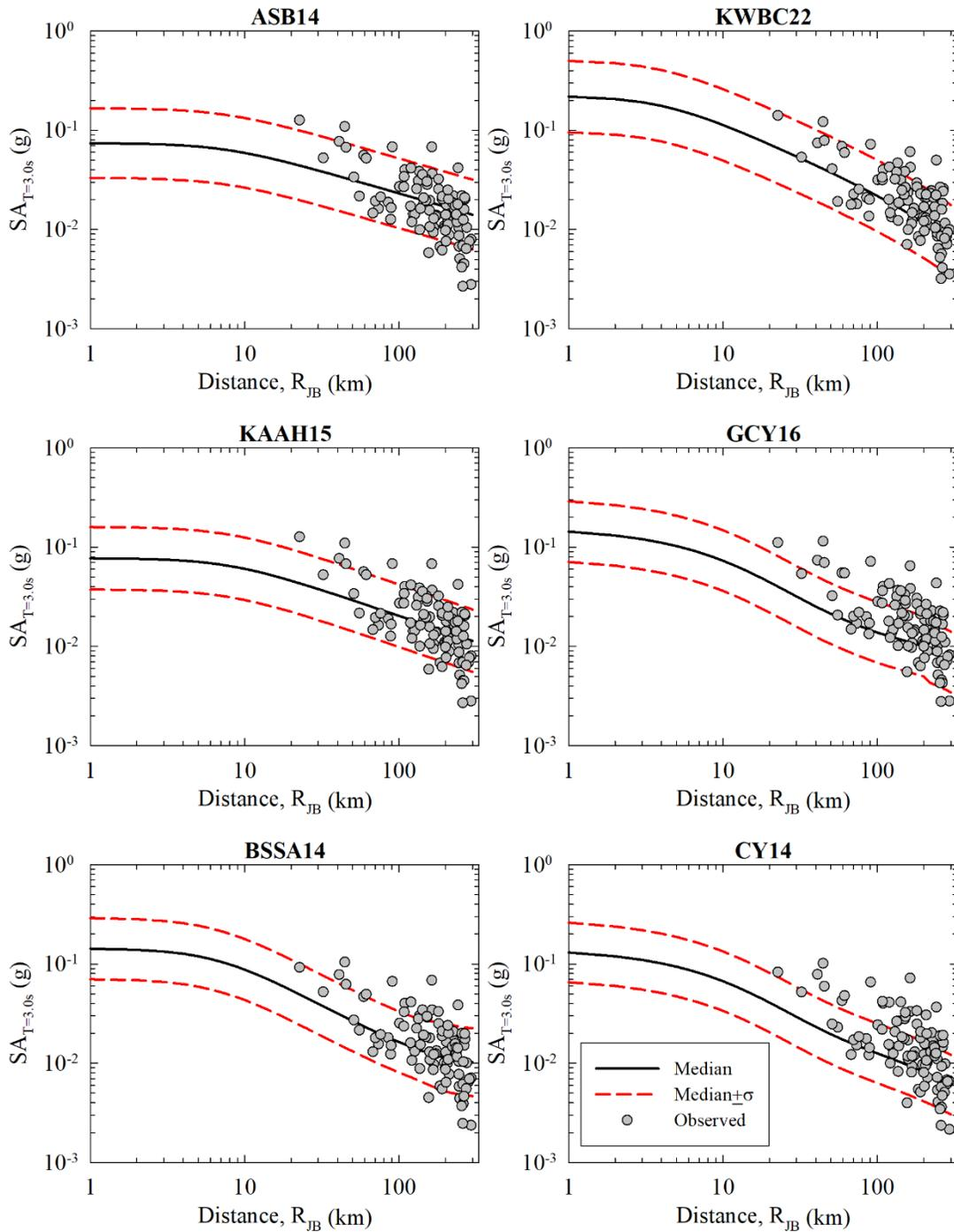
**Figure 4.26.** Comparison of the distance attenuation of ASB14, KWBC22, KAAH15, GCY16, BSSA14 and CY14 models with recorded strong motion data for  $T=3.0s$  PSA. Median and median  $\pm 1\sigma$  curves are given with black solid and red dashed lines, respectively. Gray points represent the  $V_{S30}$  normalized recorded strong motion data for Elbistan Earthquake.
