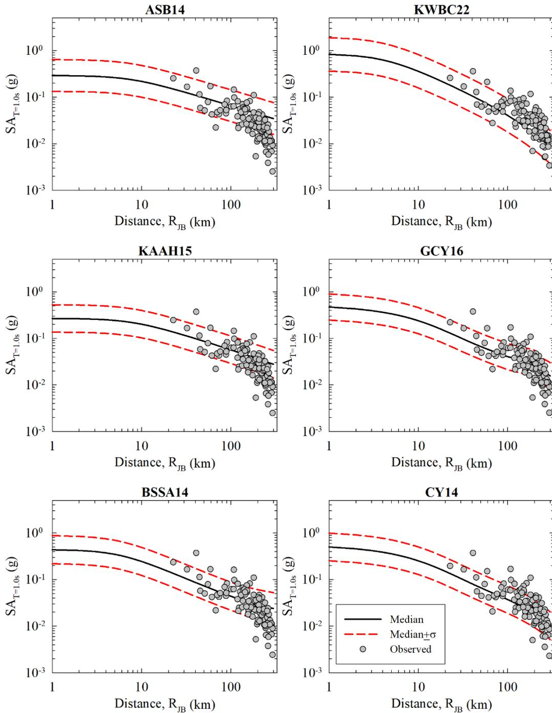
**Figure 4.25.** Comparison of the distance attenuation of ASB14, KWBC22, KAAH15, GCY16, BSSA14 and CY14 models with recorded strong motion data for  $T=1.0s$  PSA. Median and median  $\pm 1\sigma$  curves are given with black solid and red dashed lines, respectively. Gray points represent the  $V_{S30}$  normalized recorded strong motion data for Elbistan Earthquake.
