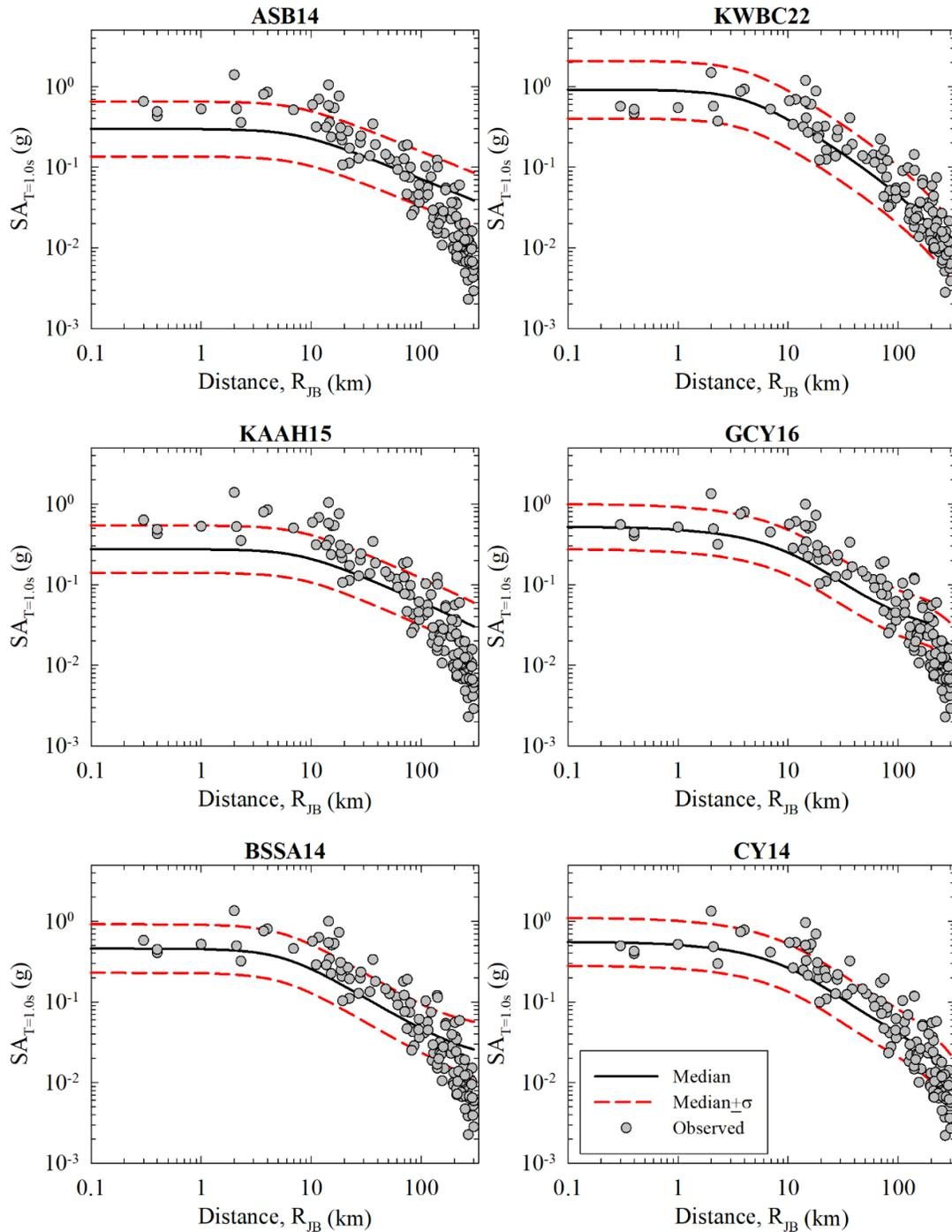
**Figure 4.20.** Comparison of the distance attenuation of ASB14, KWBC22, KAAH15, GCY16, BSSA14, and CY14 models with recorded strong motion data for  $T=1.0s$  PSA. Median and median  $\pm 1\sigma$  curves are given with black solid and red dashed lines, respectively. Gray points represent the  $V_{S30}$  normalized recorded strong motion data for Pazarcik Earthquake.
