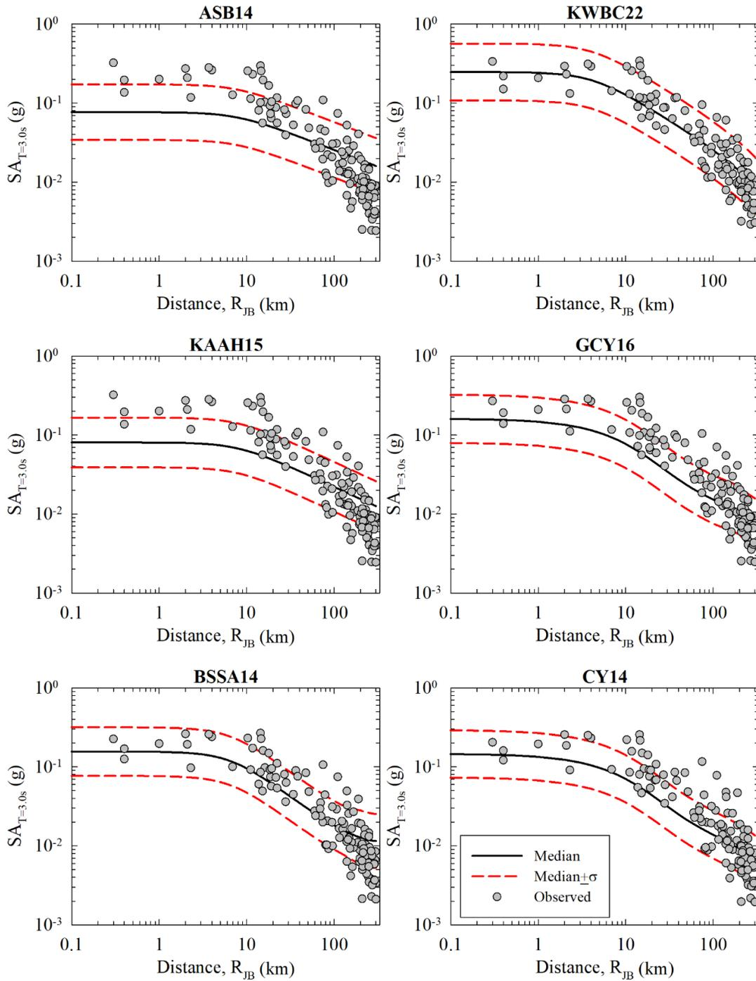
**Figure 4.21.** Comparison of the distance attenuation of ASB14, KWBC22, KAAH15, GCY16, BSSA14, and CY14 models with recorded strong motion data for  $T=3.0s$  PSA. Median and median  $\pm 1\sigma$  curves are given with black solid and red dashed lines, respectively. Gray points represent the  $V_{S30}$  normalized recorded strong motion data for Pazarcik Earthquake.
