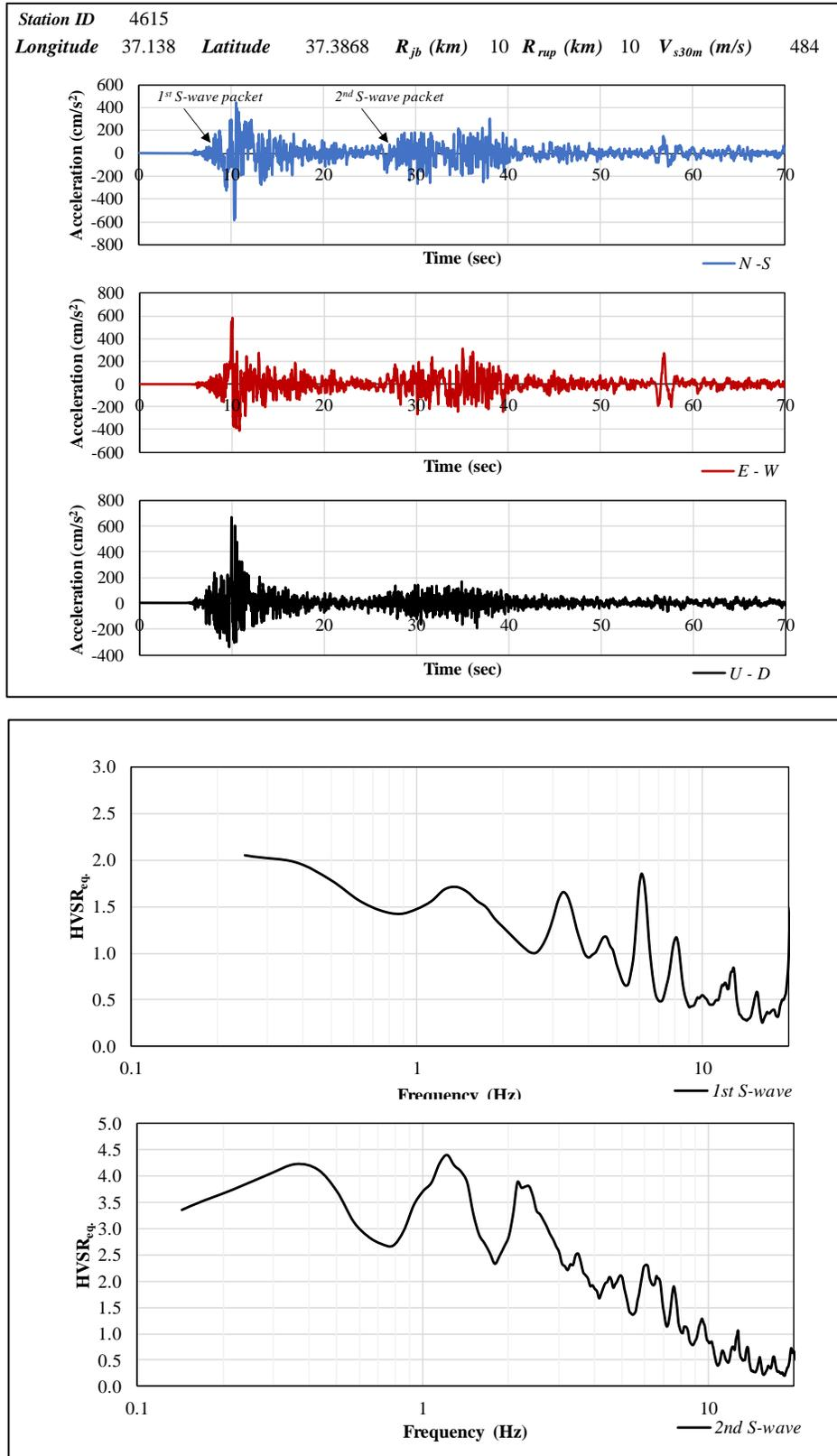
Figure 4.30. Resulting HVSR curve for station 4615
