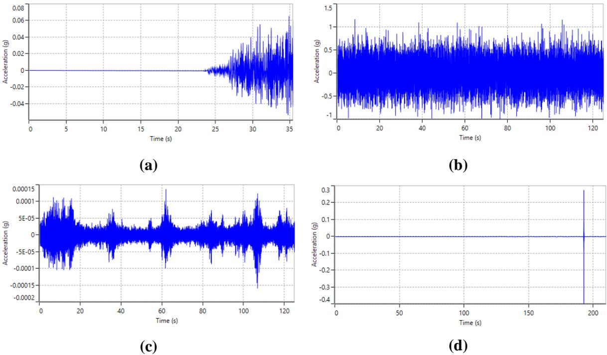
**Figure 4.3.** Samples for non-standard errors (a) incomplete trace, Station ID# 0210, (b) significant noise content, ID# 3117, (c) unclear trace of event, ID# 3113 and (d) spike, ID# 0719.
