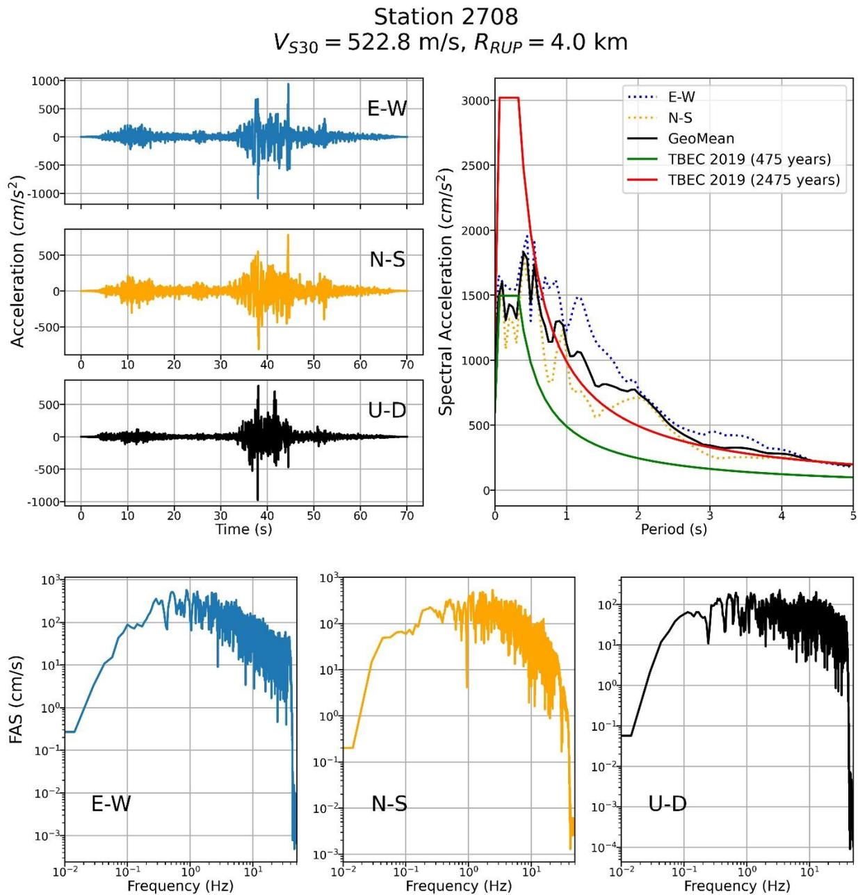
**Figure 4.8.** Recorded three-component ground accelerations, corresponding Fourier amplitude spectra (FAS) and response spectra (with 5% damping) in comparison with the most recent building code (TBEC, 2019) at selected station 2708 due to Pazarcik ( $M_w=7.7$ ) event
