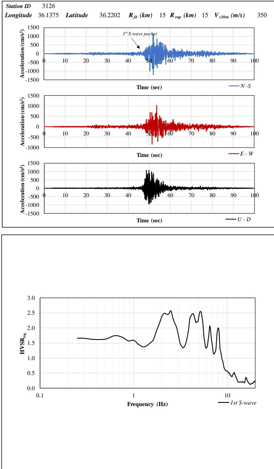
Figure 4.28. Resulting HVSR curve for station 3126
